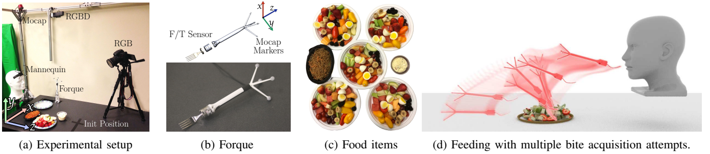
Fig. 2: Experimental setup with an instrumented fork (Forque) to acquire bites of different food items and feed a mannequin.
