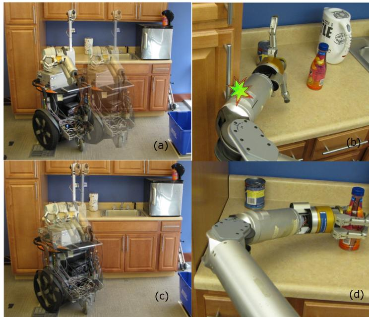
Figure 1: (a) Shows the actual pose of the robot along with a translucent overlay illustrating the estimated localized pose. (b) Due to inaccurate localization, a collision occurs at the illustrated point. (c) Real and estimated robot poses after correction. (d) Task execution with updated pose estimate.
