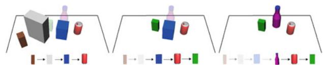
**Fig. 13** Example of replanning on a scene with two hidden objects. Each replanning stage is shown as a separate frame along with the corresponding plan. Hidden objects are shown as semi-transparent and the workspace bounds are indicated by a black line
