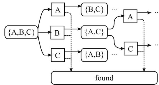
**Fig. 14** Transition graph of the of the object search MDP. States (rounded rectangles) are sets of visible objects and actions (squares) correspond to removing an object from the scene. Each action has a probability of revealing target and transitioning into found
