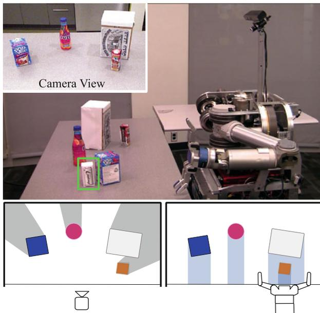
**Fig. 1** An example of the object search problem on a real robot. The robot is searching for a target object (highlighted by the *bounding box*) on the table, but its view is occluded (drawn as *gray regions*) by other objects. The robot must remove these objects to search for the target. Objects may block the robot's access to other objects
