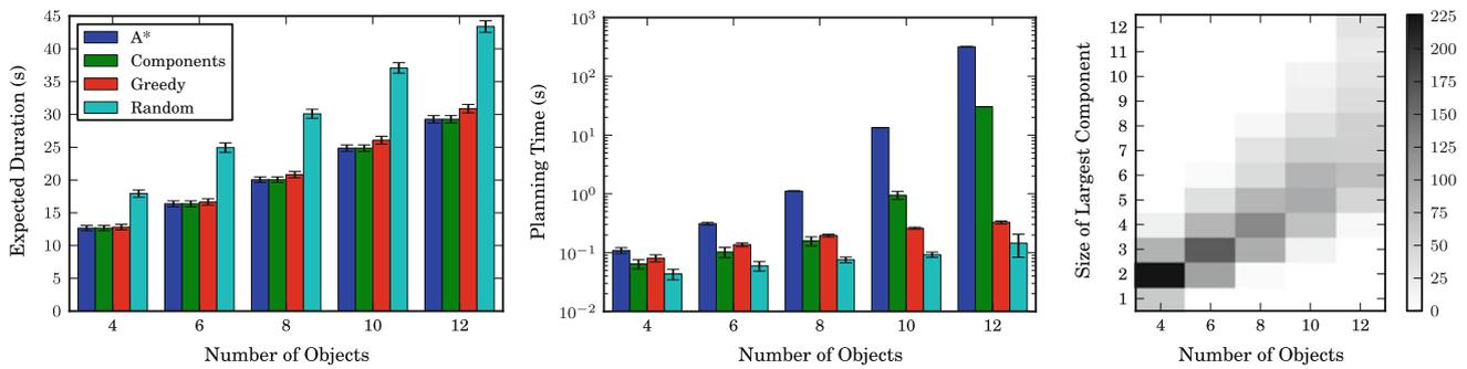
**Fig. 6** Performance of the random, greedy, A-Star, and connected component planners as a function of number of objects. All results are averaged over 400 random scenes and are plotted with their 95 % confidence interval. The planning times are presented in log-scale, where the
