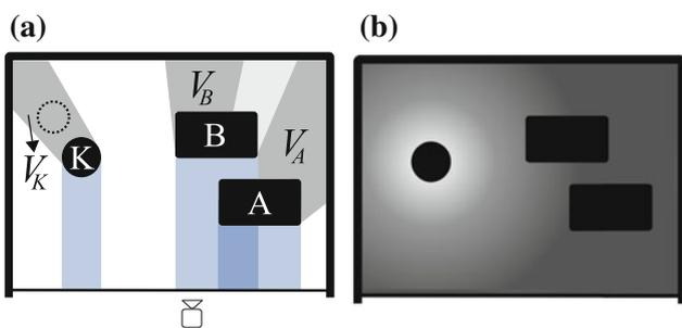
**Fig. 12** Example scene where semantic knowledge influences the optimal order of removing objects. The robot is searching for the mustard (dotted circle) and has a strong prior distribution that it is near the ketchup ( $K$ ). **a** Refrigerator scene. **b** Prior distribution  $P_0(x)$
