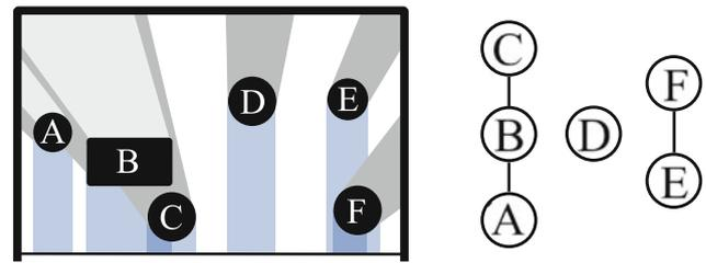
**Fig. 5** Left an example scene. Volumes occluded by a single object are shown in dark gray, joint occlusions are shown in light gray, and swept volumes are shown in light blue. Right The corresponding graph with three connected components (Color figure online)
