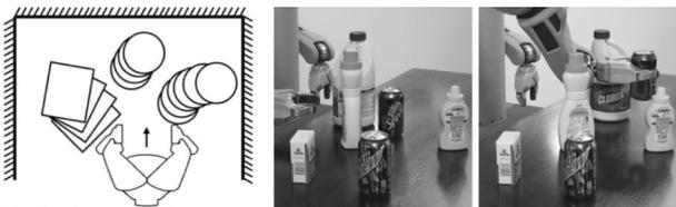
**Fig. 2** Manipulation of objects through clutter. (Left) Given a manipulator trajectory our planner predicts how each contacted object will move, and verifies that the goal will be reached successfully. (Right) An example execution, where the robot pushes two blocking objects out of the way simultaneously as it is reaching a can. Images taken from [15]
