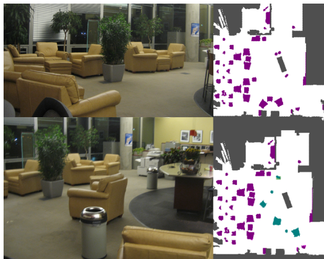
Fig. 1. A situation that requires an object based map. The top image represents the initial configuration of the map. The bottom image is the same map, with the furniture re-configured. By using an object-based map, the robot was able to rearrange the furniture in its own map to match the real world. The robot accomplished this task by noticing which objects were no longer where the static map indicated, and point-matching those objects to objects it observed. In addition, the robot labeled the moved furniture, as well as furniture in the map that looked similar, as movable.
