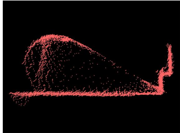
(b) The image shows the kettle standing on a table (with the handle to the left). The location of the laser scanner is to the upper left.
