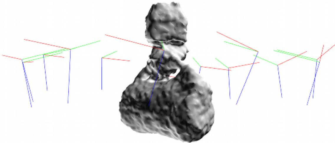
(c) The smoothed mesh of the kettle in the hand of the robot, grasping the kettle from above, with the poses of the laser scanner
