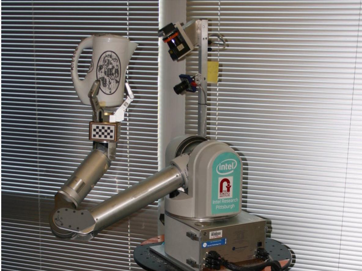
Figure 1: HERB[12] examining a novel object with its spinning laser and camera
