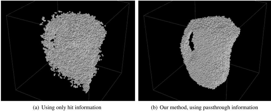
Figure 2: Our method improves the reconstruction of voxel grids from noisy laser data. This example shows the traditional method (a) and our method (b) under moderate noise conditions ( $\sigma = 5$  cm).
