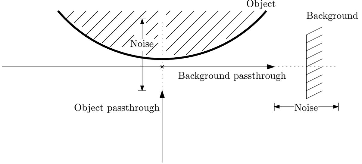
Figure 5: With noise, the hit information becomes meaningless for evaluating the occupancy of the marked point. The passthrough information from the ray passing by the object remains useful.
