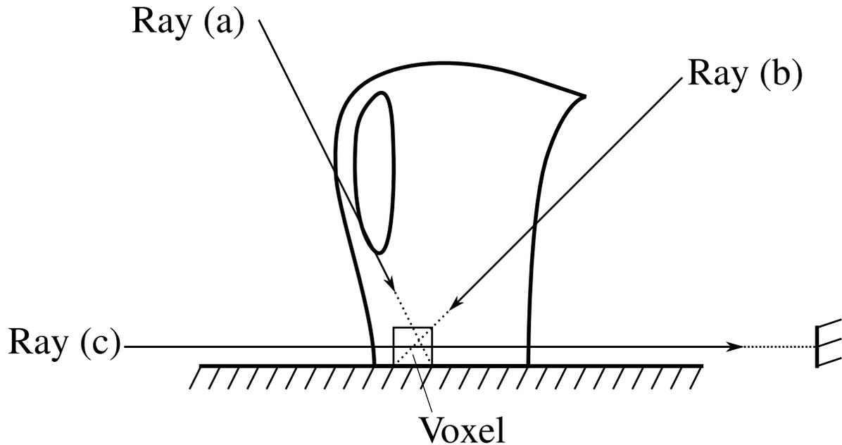
Figure 8: On Object coverage: rays (a) and (b) do not provide information about the marked voxel in the presence of noise but ray (c) does
