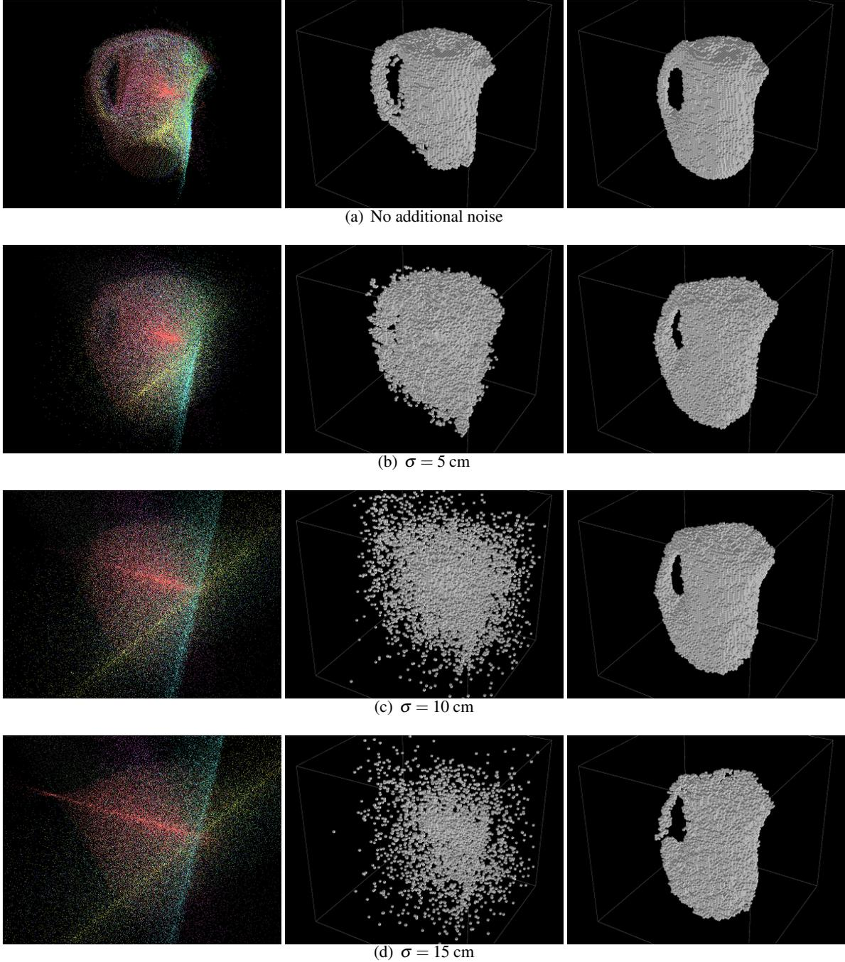
Figure 7: The effect of noisy data: the top row shows the raw point clouds. The middle row shows the result of the reconstruction using hit data only. The bottom row shows the result of our method. Our method is robust against noise, even in the order of magnitude of the object size.
