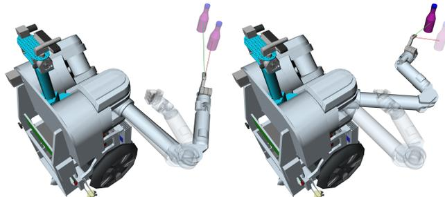
Fig. 1: Left: An efficient pointing configuration that fails to clearly convey to an observer that the goal is the further bottle. Right: Its less efficient, but *more legible* counterpart, which makes the goal clear.
