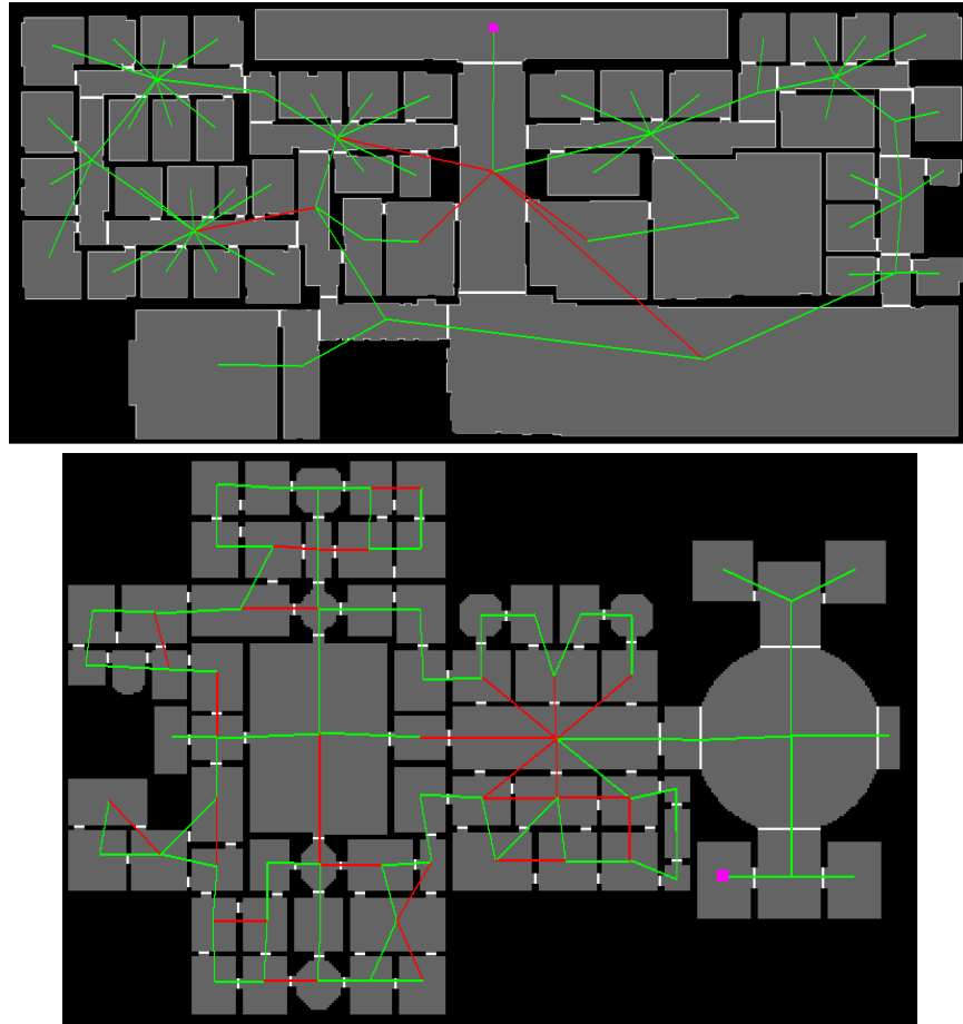
Figure 5: Example spanning trees found for the office (top) and museum (bottom) that yield minimal search schedules. The office spanning tree yields a search strategy with three searchers, and the museum tree yields one with five. Green edges denote edges in the spanning tree, and red edges denote edges that need to be guarded during search. The square denotes the searchers' starting position.
