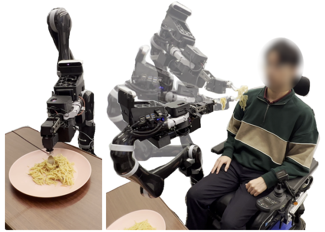
Fig. 3: The Articutool performing dynamic twirling of spaghetti during acquisition and delivering the bite for transfer.
