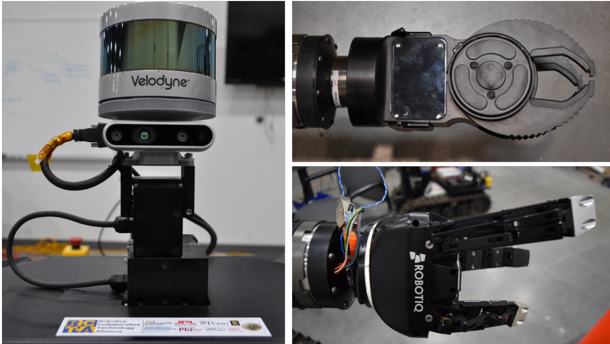
Figure 3. Sensors found within (left) head assembly and (right) selected end-effectors.
