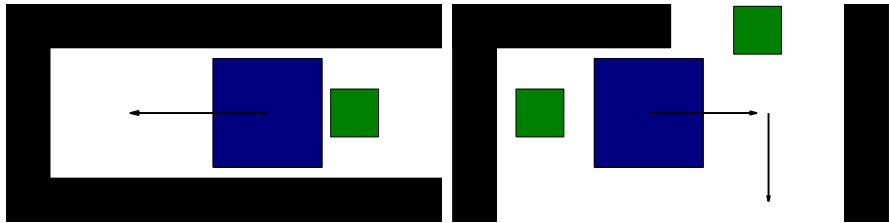
b Two feasible scenarios: (left) connected component to left of B is not required to be occupied, and (right) robot can access the top face of B to push it down.
