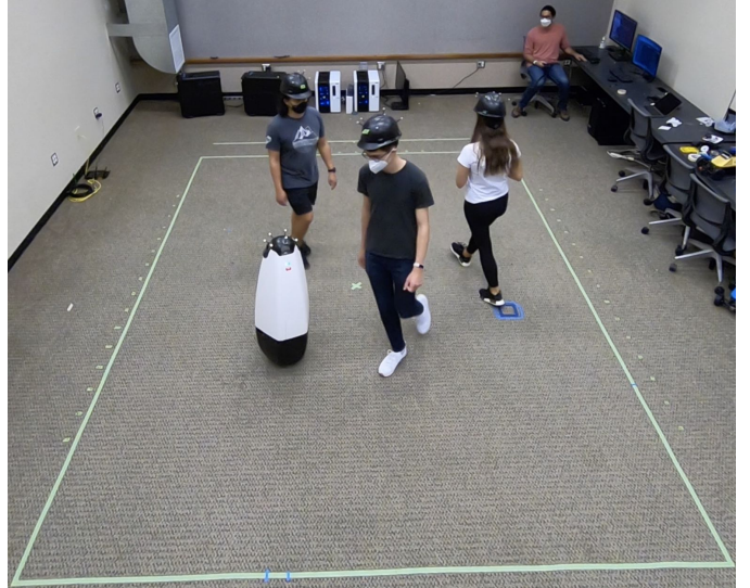
Fig. 1: Honda’s experimental ballbot [12] navigates next to three users during our lab experiments.
