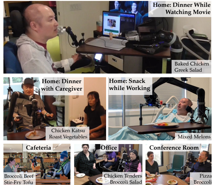
Fig. 1. We evaluate the robot feeding system with: (Bottom) an n = 5 study across 3 out-of-lab locations; (Top) a 5-day, n = 1 in-home deployment.
