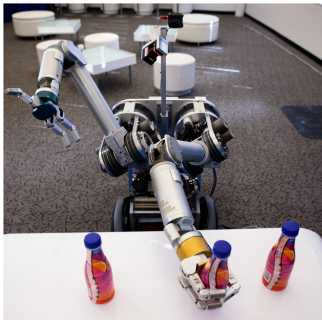
Fig. 6. HERB 2.0: A bimanual mobile manipulator developed at the Personal Robotics Lab at Carnegie Mellon University
