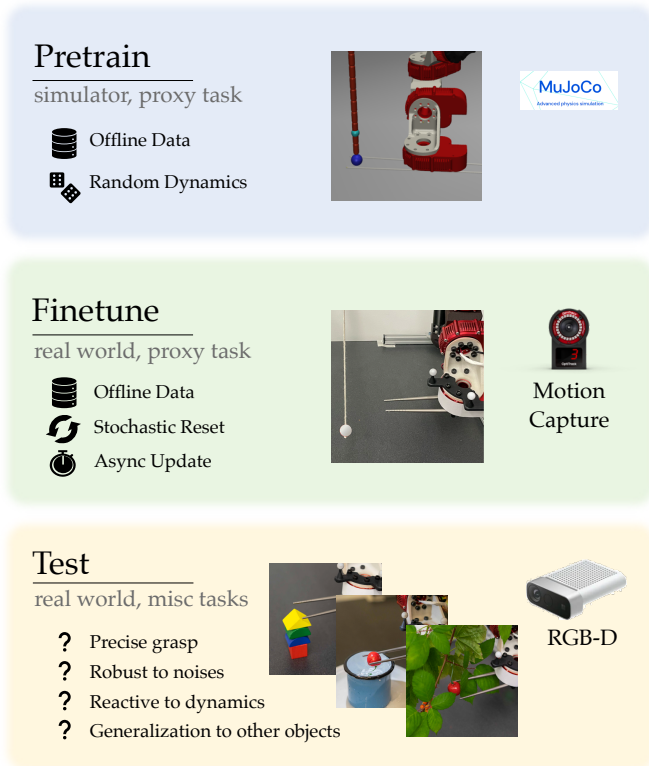
Fig. 3: An overview of the learning framework. The system first pre-trains in simulation and then fine-tunes in the real world. We carefully design the training paradigm to ensure sample efficiency and learning robustness.
