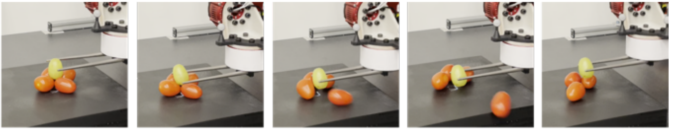
Fig. 2: The dynamic grasping task is challenging: any contact with an object might set it into motion, which is difficult to model. This challenge is exacerbated when fine manipulation is required, especially in the presence of sensor noise and perception errors.
