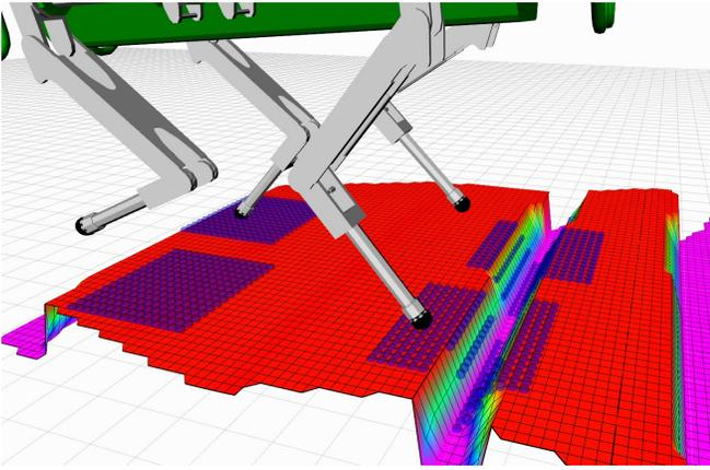
Fig. 1: Simulation of the quadruped robot HyQ collecting templates while executing a trotting gait. Templates are represented by the squared areas around future footholds, where each of the blue spheres is a potential foothold within the grid.
