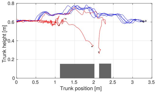
Fig. 5: Plot depicting the trunk height of the robot during multiple trials of the gap crossing scenario simulation at 0.5 m/s. Red lines indicate the trials without visual reaction activated, while blue lines indicate the trials where the visual reaction was active.
