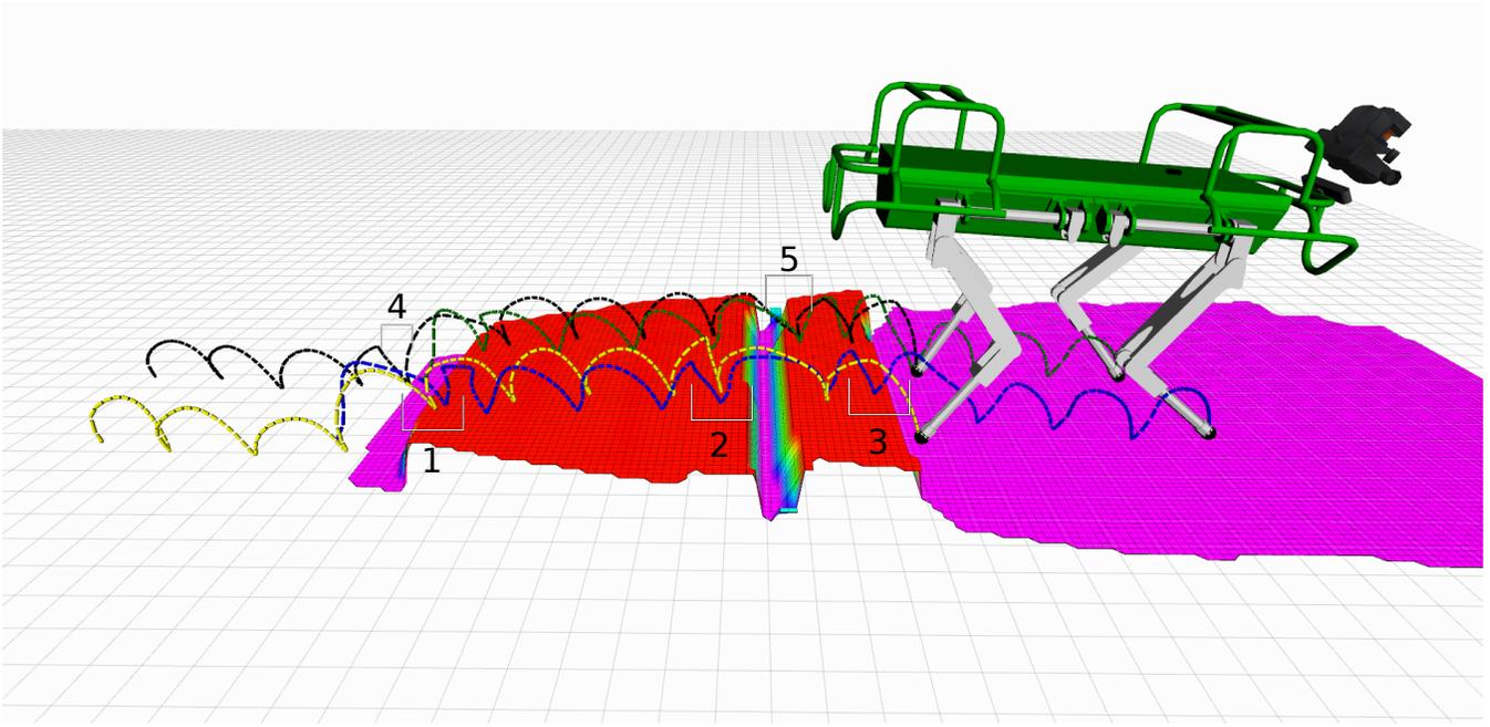
Fig. 4: Test scenario composed of a pallet with 15 cm height and 90 cm large, followed by a 15 cm height and 30 cm large wooden beam, separated by a 10 cm gap. The dashed lines correspond to the foot trajectories that are corrected by the vision-based feedback, during 0.5 m/s trotting gait: left-front (green line), right-front (blue line), left-hind (black line) and right-hind (yellow line).
