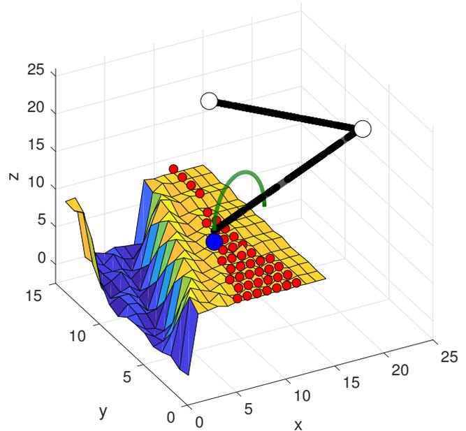
Fig. 2: Example of an evaluated terrain template. Red circles represent the set of available safe footholds, the blue circle represents the best foothold among the set of safe footholds (i.e., the closest to the center of the grid). The lower and upper limb of the leg are represented by the black solid lines and the white circles represent the location of the joints. The foot follows the trajectory indicated by the solid green line.
