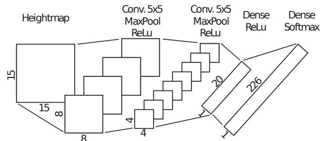
Fig. 3: Architecture of the trained CNN used to map terrain templates to foothold corrections.
